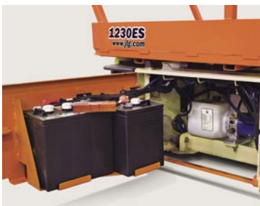
All-steel swing-out battery doors with heavy-duty hinges.
